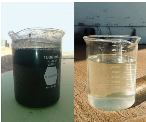
F&A's DAF effluent before and after treatment with nanobubbles.
